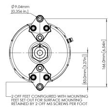
BASE CONFIGURED WITH MOUNTING FEET SET OUT FOR SURFACE MOUNTING
